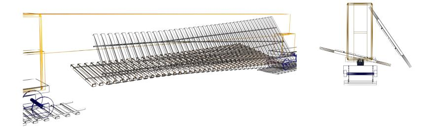
• The old block shall be put vertically and backed out to the opposite wall of the tunnel
