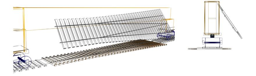
The new track switch block brought shall be backed out to the tunnel wall
