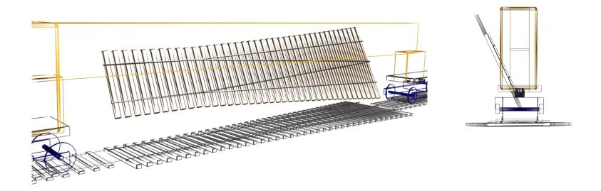
The machine shall be set to transport position and sent to the nearest station
