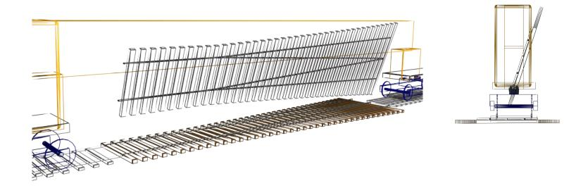
The machine brings the first block of the track switch
